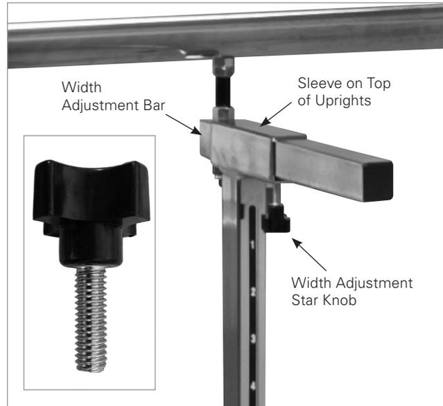
3. Adjust the height of each handrail with the spring-loaded plunger on each upright. Height is selected with the help of the number indicator strip. After adjusting the plunger, tighten the star knob next to the plunger on the upright. Repeat the process for all uprights.
