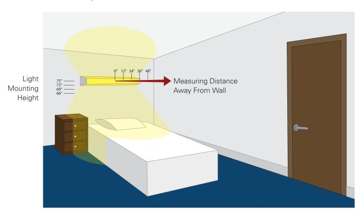
Foot-candles are measured at 66", 69", 72" and 75" heights and 0", 12", 24", 36" and 48" away from the wall. Three measurements at each height and distance are taken for the uplight, downlight and up/downlight combination.
