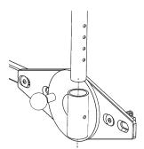
Position the assist at the desired height setting and then secure the assist with the included retention hardware.
