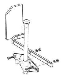
6. Insert the assist handle into the support tube on the assist device mounting plate.
