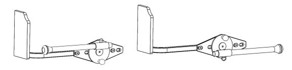
3. Adjust handle height by removing the release pin or bolt, moving the handle to the desired position, and then reinserting pin or bolt.
