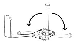
4. Set the pivot lock by inserting one or two set screws into the pivot lock holes in the back of the assist device mounting plate. See chart below for placement instructions:
