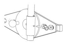
For quick-release adjustment of handle height and quick removal of the assist handle, use the included retention pin.
