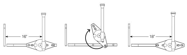
**△ WARNING:** Do not use the Direct Supply Zero Opening Assist Device if the slots do not align with your bed's assist device mounting holes.
