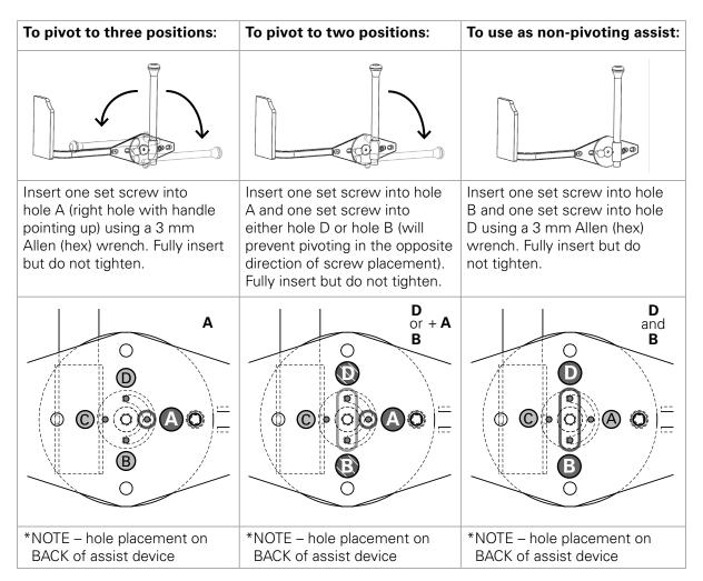
**WARNING:** Do not allow the assist device to pivot in all four directions. Allowing the device to pivot toward the floor may potentially create a crush hazard and/or damage to your bed.
