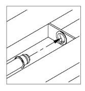
Fully insert the Side Rail Attachment Pin through the inner mount clip on the bed sleepdeck. Install (1) E-ring in the groove farthest from the side rail, 2 places per rail. When installed correctly, an E-ring should be on both sides of the sleepdeck inner mount clip. Verify that all E-rings are properly seated.
