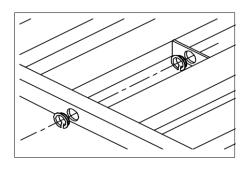
2. Insert Side Rail Attachment Pins into bed sleepdeck mount holes ensuring that the rail is properly located on the bed. Install (1) E-ring in the groove closest to the side rail on each Attachment Pin, 2 places per rail.
