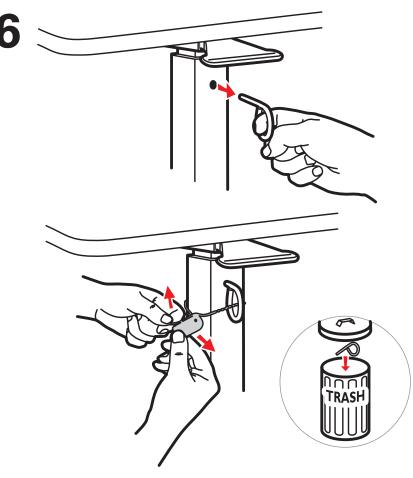
**△ WARNING:** This overbed table contains a high-tension spring-loaded system.
