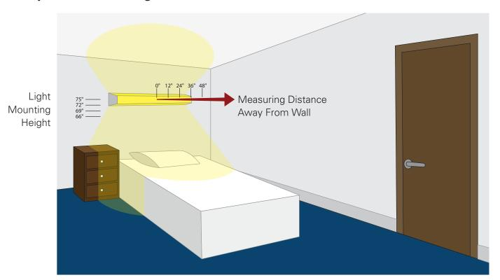
Foot-candles are measured at 66", 69", 72" and 75" heights and 0", 12", 24", 36" and 48" away from the wall. Three measurements at each height and distance are taken for the uplight, downlight and up/downlight combination.
