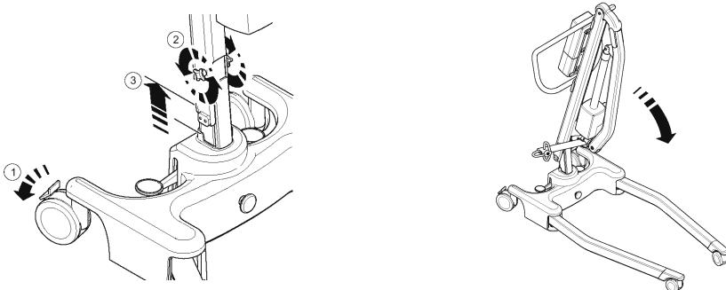
4. Lift the folded Advance upright (using the legs and push handle as a guide) being careful that the mast and boom stay together as you tilt upright.
