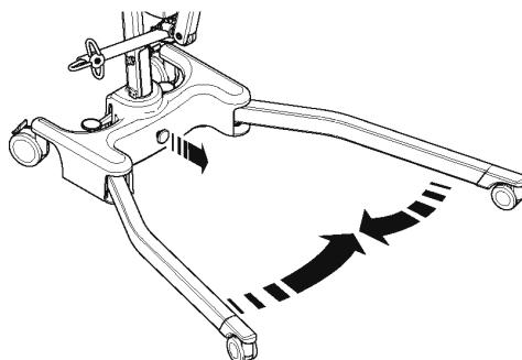
3. Loosen mast locking device (2 - not fully) lift the mast and boom assembly (3), and fold carefully toward the legs. Use the push handle to assist this motion.
