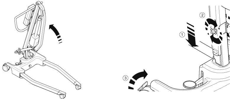
5. Open legs fully. ENSURE leg-locking knob inserts flush against the base casting and the legs will no longer move freely. The legs will then only operate by the use of the foot pedal mechanism located at the rear of the base.
