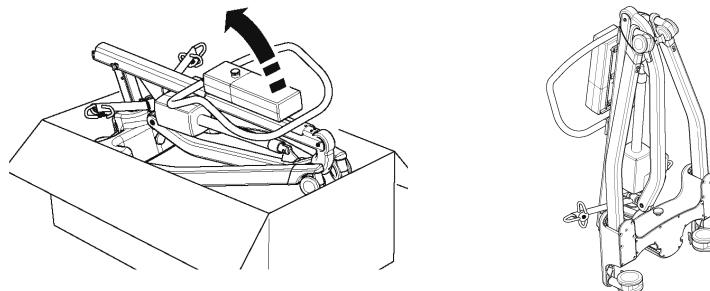
2. Release the leg and mast assembly by unfastening the restraining strap from the wheels. This strap will retract neatly into the top of the mast section.
