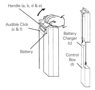
**NOTE:** The battery mounts to the control box and battery charger as shown.
