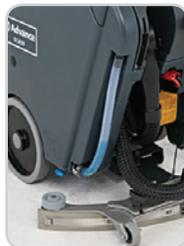
Solution drain hose also functions as the solution level indicator while large recovery drain hose offers soft, squeezable section to enable manual flow control.
