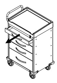
2. Push release levers in middle of both slides, one up and one down.
