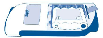
**NOTE:** Be sure to insert the battery pack in the proper positive/negative orientation or the unit will not operate.
