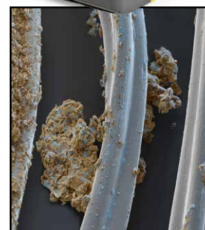
Magnified view of iCapsol™ encapsulating cleaning technology at work. Left = dirty, Middle = encapsulated soil, Right = cleaned with iCapsol.
