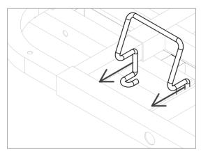
2. Push the mattress retainer onto the deck.
